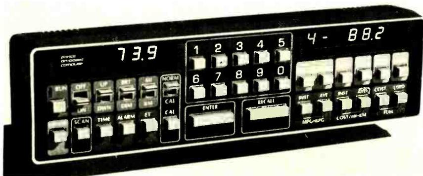
**AUTOMOTIVE COMPUTER** provides motorists with a driver controlled information center with 24 functions. At a touch of the button, vehicle location, trip information, time of day and fuel economy data can be displayed on the LED digital display. The unit is expected to retail for \$400.
