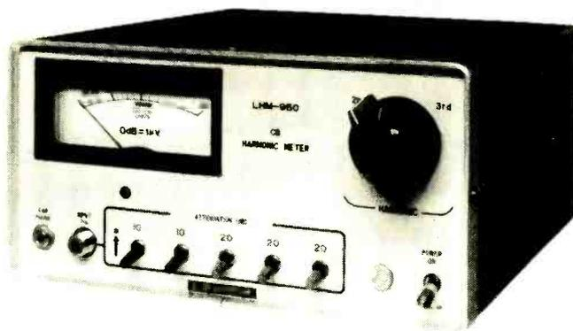
*Many television interference complaints are caused by the second and third harmonics from CB transceivers. A special test instrument has been developed so technicians can easily measure interference components.*
