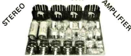
OCL pre amp. & power stereo amp. with bass, middle, treble 3-way tone control. Fully assembled and tested, ready to work. Total harmonic distortion less than 0.5% at full power. Output maximum is 60 watts per channel at 8Ω. Power supply is 24 - 36V AC or DC. Complete unit
