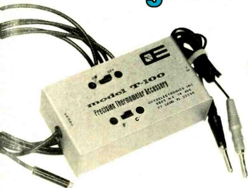
*A simple, easy-to-build accessory converts your digital voltmeter into a handy thermometer for monitoring semiconductor case temperatures, photographic chemicals and numerous other uses around the lab, home and workbench.*
